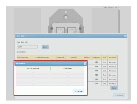
This window displays the Device Names you set in "Device Settings" section.
