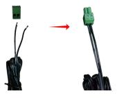
Plug in the 2-pin cable equipped phoenix connector to DC 12V port of the keypad. Connect the adapter to the power, the keypad should start work(press the any button, it will flash).
