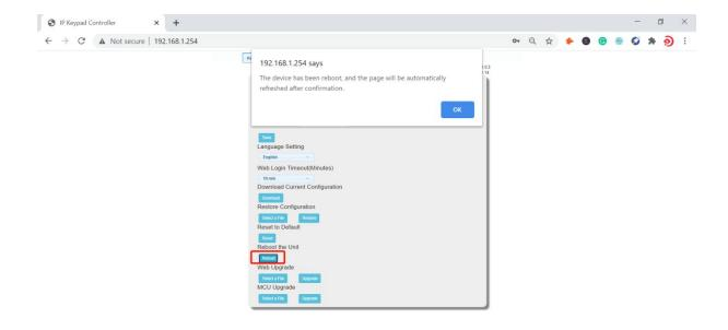
After rebooting the keypad successfully, the buttons on front panel blink 3 times and the web page returns to the login page.
