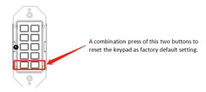
\* Press the two buttons shown in the above picture at the same for at least until all the backlights of the buttons blink 3 times, the keypad will be reset to factory defaults.
