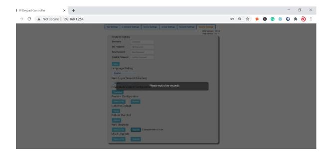
When web UI upgrading is completed, the keypad will reboot automatically and the web page will be refreshed automatically.
